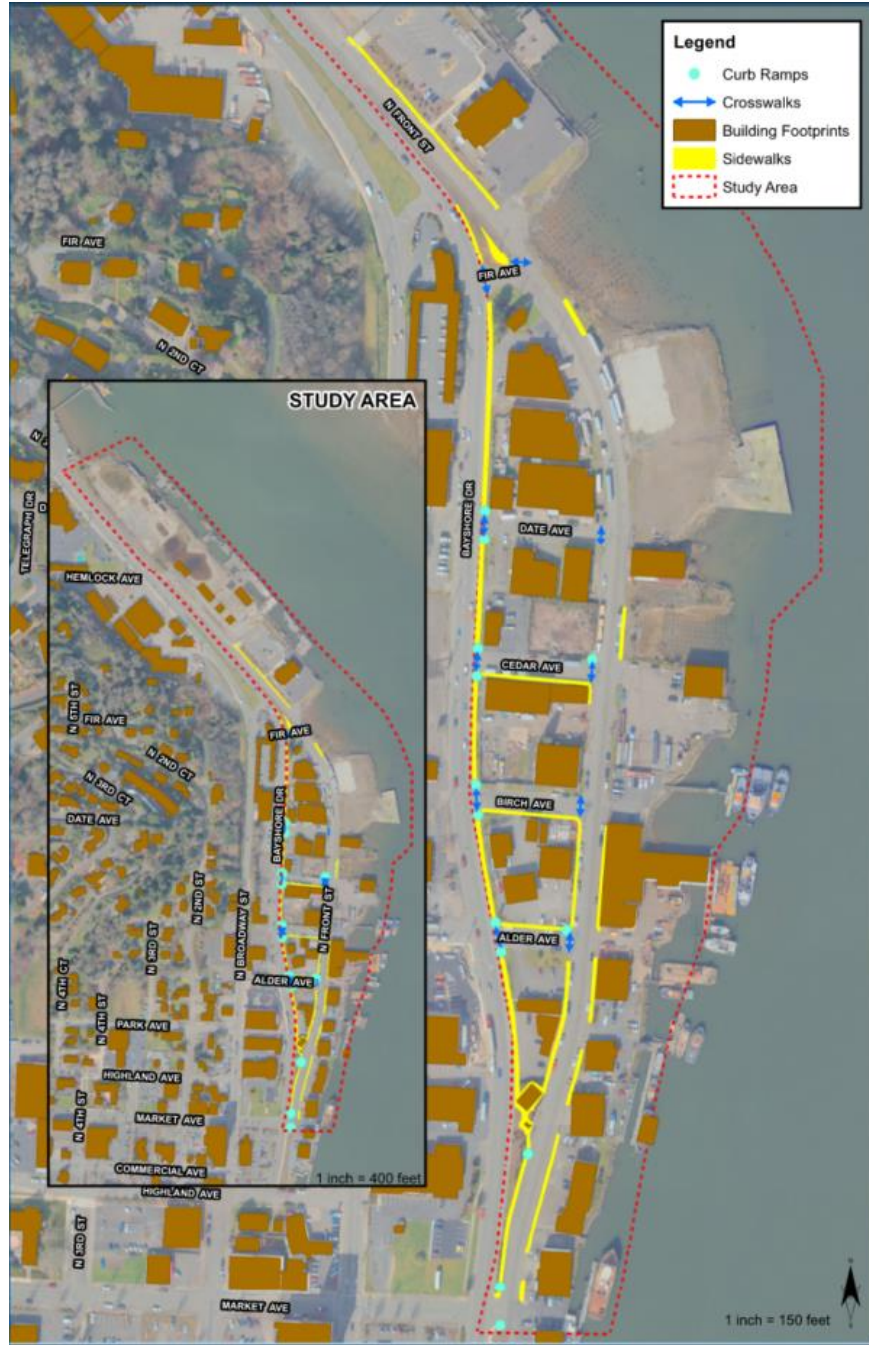
Figure 5. Sidewalk, Crosswalk, Curb Ramp Inventory
